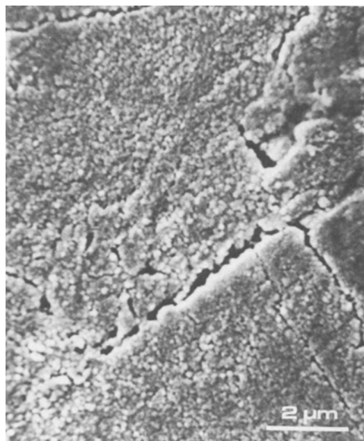
Figure 6 Scanning-electron micrograph of a cross section of a nitrided (90 h; 10 vol % \text{NH}_3 /90 vol % \text{H}_2 ; 803 K) FeCrC (3.16 wt % Cr; 0.20 wt % C) specimen (H-structure; depth below surface 40 μm). On prolonged nitriding, voids develop at grain boundaries.
