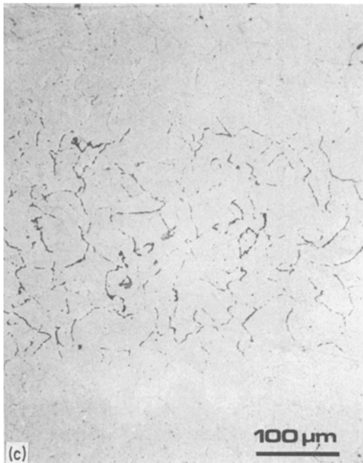
Figure 2 Optical micrographs of the entire cross sections of nitrided (a: 7.5 h, b: 20 h, c: 48 h; 10 vol % \text{NH}_3 /90 vol % \text{H}_2 ; 803 K) FeCrC (3.16 wt % Cr; 0.20 wt % C) specimens (A-structure). During nitriding carbide-rich zones move to larger depths below the surfaces (carbides stained by Murakami etching).
