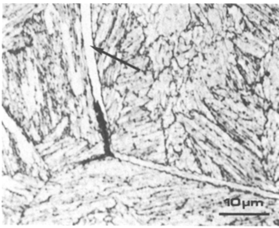
Figure 7 Optical micrograph of a cross section (nital etched) of a nitrided (210 h; 10 vol % \text{NH}_3 /90 vol % \text{H}_2 ; 803 K) FeCrC (3.16 wt % Cr; 0.20 wt % C) specimen (QT-structure) showing a channel in open contact with the surface. Note electrolytically deposited nickel in that channel (arrow; top of figure coincides with surface).
