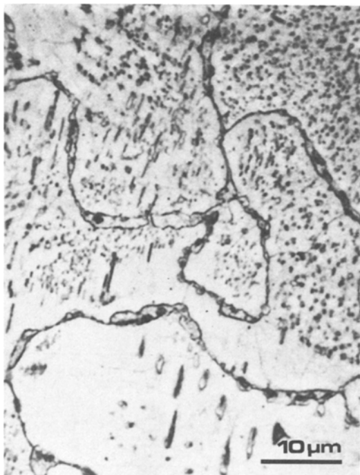
Figure 4 Optical micrograph of a cross section (Murakami etched) of a nitrided (210 h; 10 vol % \text{NH}_3 /90 vol % \text{H}_2 ; 803 K) FeCrC (3.16 wt % Cr; 0.20 wt % C) specimen (A-structure; depth below surface 250 μm), showing regions along grain boundaries transformed by a discontinuous precipitation reaction.
